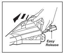
5. Carefully insert and twist screwdriver at each brush support to free brush from base.
